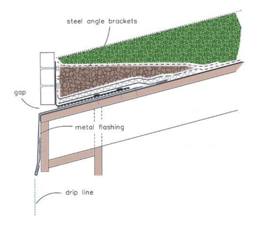
*Example eave detail for sloped roof* Source: Roofscapes, Inc.
