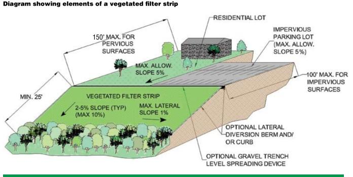
slope needs to be determined. This information is used to determine the length of the filter strip using the appropriate graph (Figures 7.52 through 7.56).
