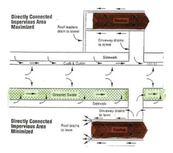
Difference between maximizing and minimizing runoff Source – Center for Watershed Protection
