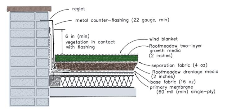
*Example parapet flashing detail for a flat roof* Source: Roofscapes, Inc.
