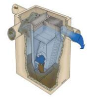
*Vortex Hydrodynamic Separator* Source: Stormwater Solutions
