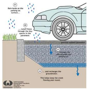
Pervious pavement with infiltration schematic
