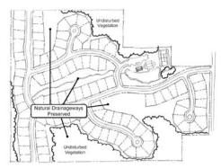
Schematic of a site design protecting natural drainage features Source: Georgia Stormwater Management Manual, Volume 2: Technical Handbook, First Edition. August, 2001
