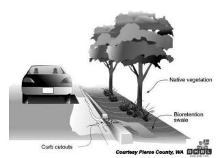
*Curb cut-outs allow stormwater runoff from a parking lot to flow into a bioretention swale* Source – Pierce County, WA and RHBL
